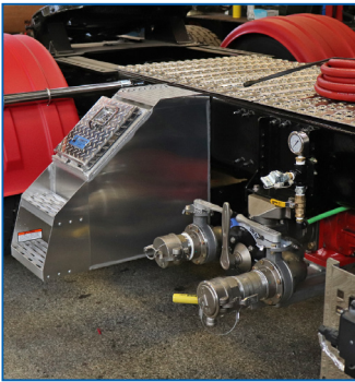
Flow Control System Mounted on Tank or Truck to connect to PTO (drive-line or hydraulically)
